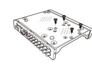
a) Connect the data and power cables to the HDD and place the HDD on the DVR case.
