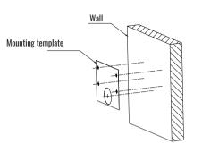
Step 1:Stick the mounting template to the wall, drill 4 screw holes and 1 tail cable hole.
