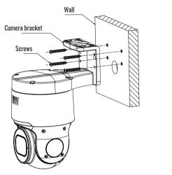
Step 3:Align the camera bracket with the 4 swelling colloidal particles screw holes, and lock the screws to fix it
