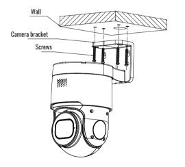
Step 3: Align the camera bracket with the 4 swelling colloidal particles screw holes, and lock the screws to fix it.
