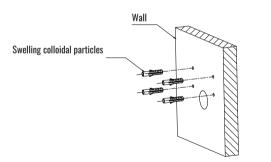
Step 2: Hammer the 4 swelling colloidal particles into the drilled wall holes.
