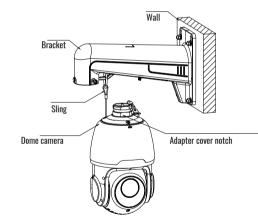
Step 6: After rotating the dome camera to the proper position, tighten the 2 socket head cap screws M6\*16 on the bracket.
