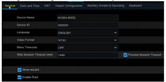
Note: After the RAID function is enabled, the NVR does not support ESATA and NAS.
